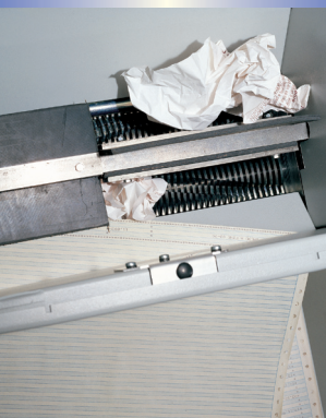
Automatic mechanical feeding system with revolving flaps
